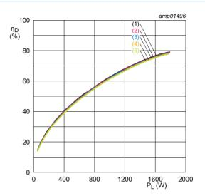
$V_{DS} = 55 \text{ V}$ ; f = 108 MHz;  $t_p = 100 \text{ }\mu\text{s}$ ;  $\delta = 10 \text{ }\%$ .
