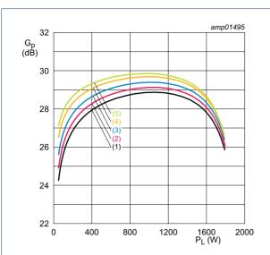
$V_{DS} = 55 \text{ V; } f = 108 \text{ MHz; } t_p = 100 \text{ } \mu\text{s; } \delta = 10 \text{ } \%.$
