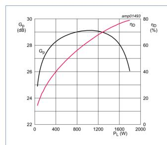
$V_{DS}$  = 55 V;  $I_{Dq}$  = 100 mA per section; f = 108 MHz;  $t_{D}$  = 100  $\mu$ s;  $\delta$  = 10 %.
