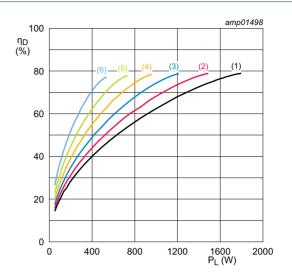
$I_{Dq}$  = 100 mA per section; f = 108 MHz;  $t_p$  = 100  $\mu$ s;  $\delta = 10 \%$ .
